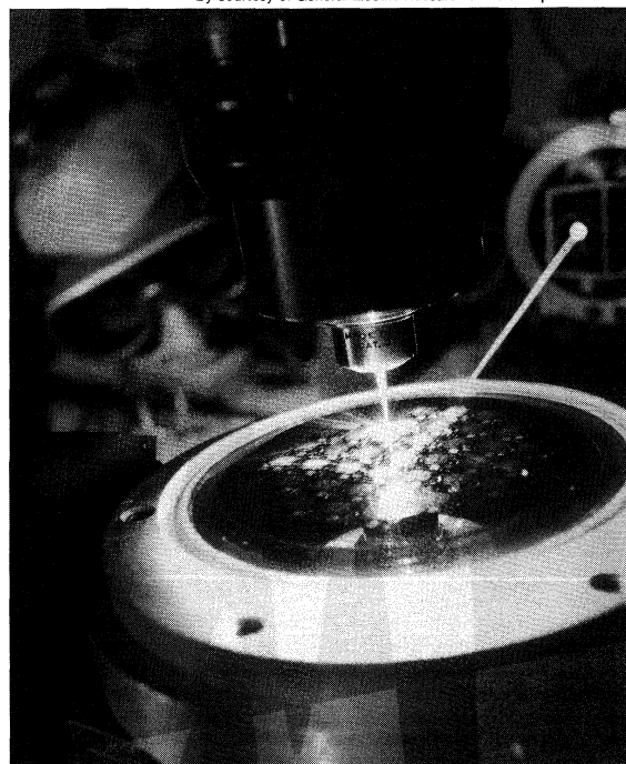
Figure 9: A laser scribing microscopic lines that connect integrated circuits.
